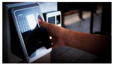
Another critical area where biometrics are making an impact is in physical security. A biometric access control device allows only authorized individuals to enter restricted areas, enhancing the overall safety of offices, factories, or residential complexes. These devices can also be integrated with attendance systems to provide a comprehensive security and time-tracking solution. Sathya Online Shopping stocks the latest access control devices with high durability and performance.
